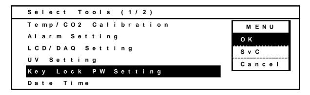
**3.** Input the current user password (4 digits), select **OK**, and press the ENTER Key. (The default user password is 0000 when the Incubator is shipped from the factory.)
